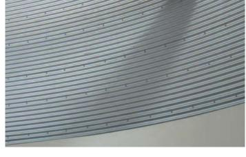
This panel has 37 ¼" wide coverage and can be curved convex, concave, horizontal or vertical. Convex and concave styles are machine curved. Vertical styles are simple wrap-arounds, overlapping or nesting at sides. Contact ATAS for horizontal curving applications.
